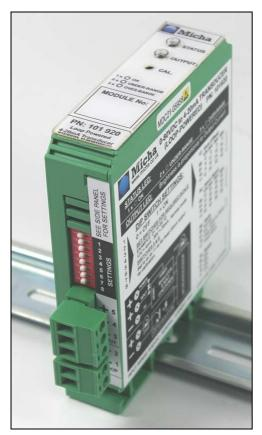
The **Micha Battery Voltage to 4-20mA Transducer** (PN: 101920) has been designed for use in any application where a 4-20mA signal is required from a DC voltage source. The control circuitry is powered from the input and, as a loop-powered device, it requires a suitable current source to be connected to the output.
