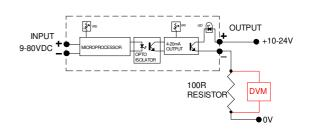
Note: if the input voltage exceeds the Span setting, the output will remain at the maximum of 20mA but the STATUS LED will flash three times.
