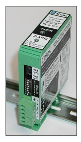
The **Micha** Battery Voltage to 4-20mA Transducer (PN: 101920) has been designed for use in any application where a 4-20mA signal is required from a DC voltage source. The control circuitry is powered from the input and, as a loop-powered device, it requires a suitable current source to be connected to the output.
