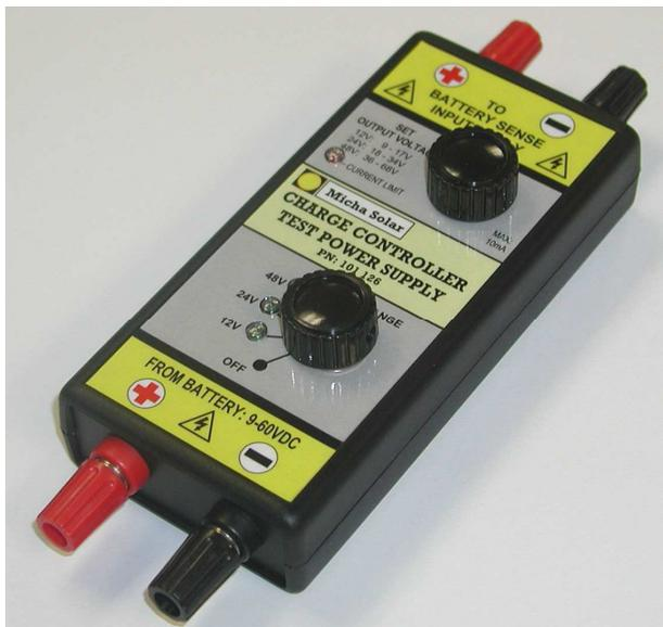
The **Micha Test Power Supplies** have been designed to assist in the commissioning of the MSR<sub>x</sub> range of solar charge controllers, as well as any other similar application where a portable and variable low power voltage source is required.
