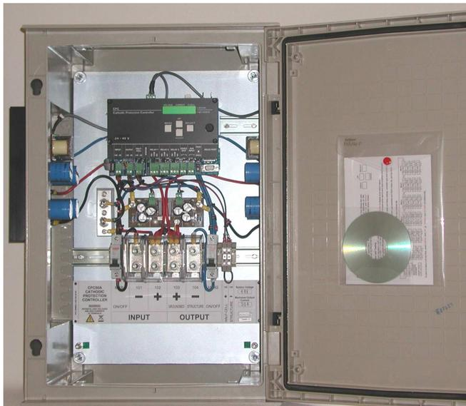
The CPC25A and CPC50A are part of the new generation of Cathodic Protection Controllers, which feature microprocessor control, three programmable alarm/function relays, built-in interrupt timer, and an RS232 Port with Data Logging as standard.
