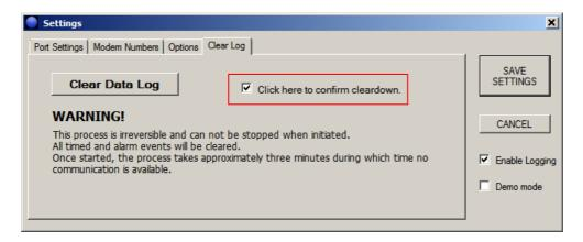
To start the data cleardown, tick the confirmation box and then click on 'Clear Data Log'. During cleardown, all communications with the MSRx controller is disabled.
