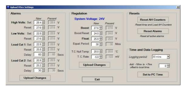
**Alarms**: The Set and Reset voltage settings can be changed for the High Volts and Low Volts alarms, as well as the Disconnect, Reconnect and Delays for Load Cut 1 and Load Cut 2.
