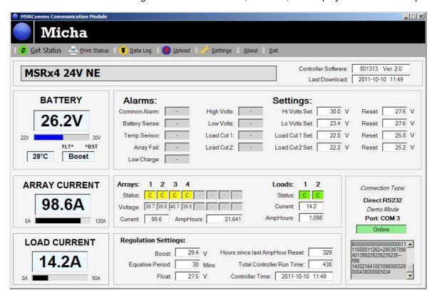
The bargraph below the Battery voltage has markers for the Float and Boost settings allowing a quick evaluation of the battery status and this panel also displays the measured Battery temperature, and present regulation mode.
