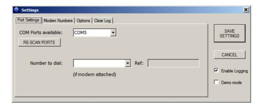
Click on **RE-SCAN PORTS** and all available RS232 ports should be detected. Select the appropriate port from the drop-down box, e.g. 'COM4', and click on **SAVE SETTINGS**. If a modem is detected, the this will be indicated with (M) shown as 'COM4 (M)'. Up to five modem numbers can be entered by clicking on the 'Modem Numbers' tab - these will then available for selection in the 'Number to dial' drop down box.
