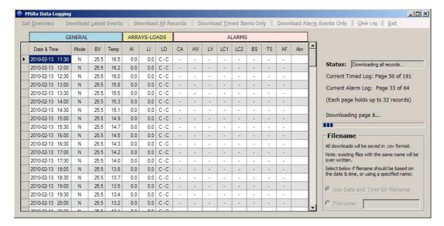
Once a download has been made, the data is displayed in table format as above and can be sorted by various categories by clicking on the column header. For example, to sort the data by Battery Voltage, click on the 'BV' header.
