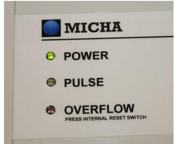
The **Micha** 8-Input Pulse Combiner/Divider unit is designed to allow the integration of pulses from multiple energy meters into a single, controlled stream to give a single connection to a Power Generation Display Unit. In addition, the combined pulse rate can be divided by factors of 5, 10, 20 and 40, to reduce the total output pulse frequency.
