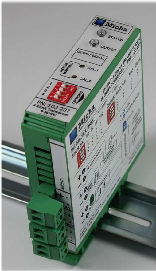
The **Micha** range of **Shunt to 4-20mA Transducers** have been designed for use where a 4-20mA signal is required from a 50mV, 60mV, 75mV or 100mV shunt. The modules come in two supply-voltage versions: one will operate from 9VDC to 36VDC and the other from 18V to 65VDC. (See the table at the end of the datasheet for part numbers.)
