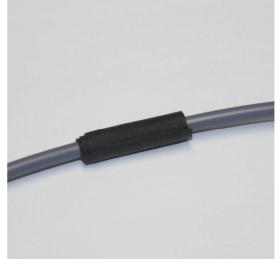
Wrap the tape around the cable in the position where it will pass through the cable gland. The tape should be slightly stretched as it is applied to ensure it bonds to itself. Complete wrapping the tape around the cable until an appropriate final diameter is obtained, and stretch the end to produce a smooth finish. Pass the connector end of the antenna lead through from the outside of gland and tighten.
