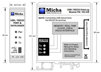
The **Micha** RS232 and USB Port (PN **102 438**) is a combined Port and Datalogger and replaces previous versions 101595 and 101596. The module allow the end user to directly communicate with the controller via a USB port or RS232 port on a PC or laptop. The module allow 'snapshots' of the current status to be downloaded and displayed, and the Data Logger has the ability to log the status at 15, 30 or 60 minute intervals, allowing in excess of two months of historical data to be stored.
