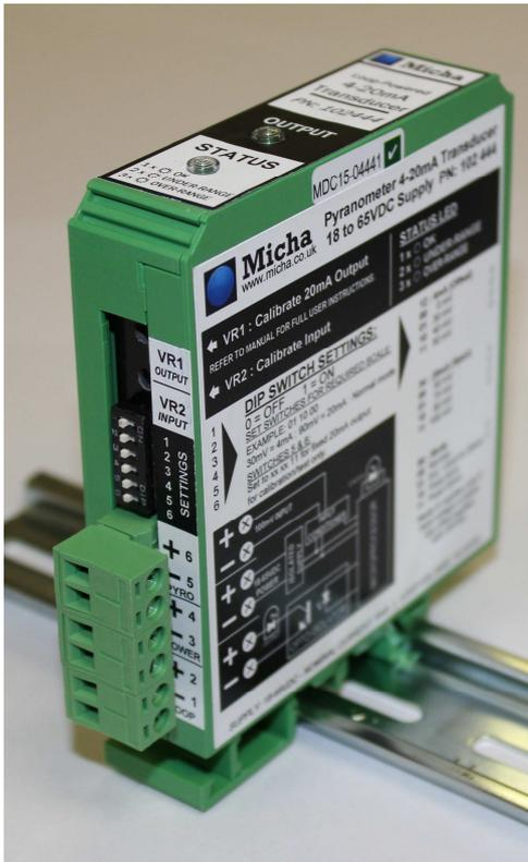
The **Micha Pyranometer to 4-20mA Transducer** has been designed to be used in conjunction with Pyranometer PN 102 443 which has a nominal output of  $95\text{mV} \pm 8\%$  at  $1000\text{W}/\text{m}^2$
