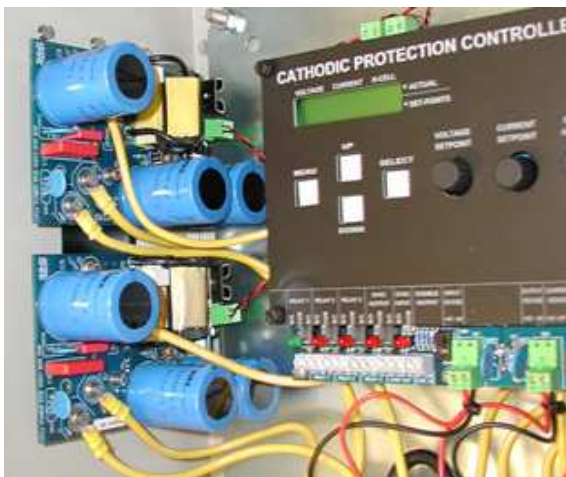
Two 400946 CPCx 25A Power PCB Assemblies installed in a CPCx50A Controller (Painted Steel enclosure)
