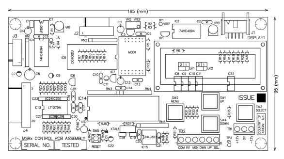
PCB Assembly Name: MSRx Control PCB Assembly V1 ext. switch inputs
