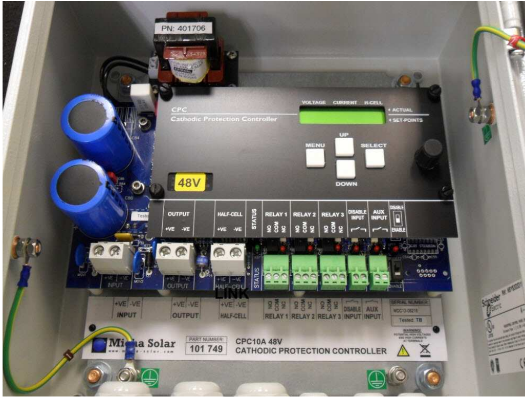
Above: CPC10 48V V1 with no RS232 port. PN 401706 shown top left
